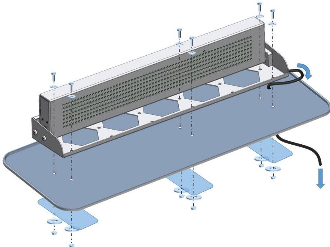
**PREVOIR DES CONTREPLAQUES ADAPTEES (NON FOURNIES) AU SUPPORT ENTRE LA PLAGE ARRIERE ET LES GROSSES RONDELLES / PLAN APPROPRIATE MOUNTING PLATES (NOT SUPPLIED) BETWEEN BIGGEST WASHERS AND MOUNTING PLATE.**
