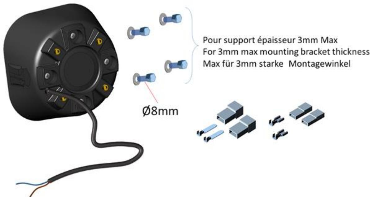
**! LE HAUT-PARLEUR DOIT ETRE INSTALLE AVEC 4 VIS / ! LOUDSPEAKER MOUNTING WITH 4 SCREWS / LAUTSPRECHERMONTAGE MIT 4 SCHRAUBEN**
