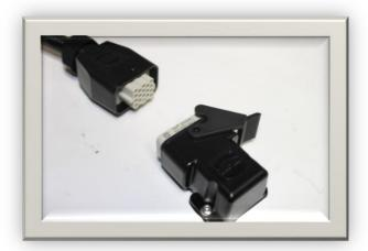
New generation roof connector, for maintenance and transfer to another vehicle.
