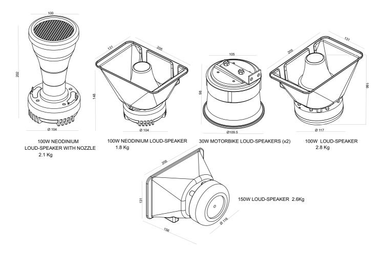
NOTE: The siren flash module is designed and approved for functioning with one of the five loud-speakers described Above. The power obtained varies according to the loud-speaker model chosen.
