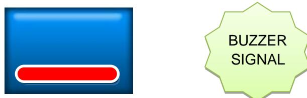
Press a second time on the button to control the function again. If the fault disappears, the band becomes green and the audio warning stops. If the fault is still present, the alarm will appear again.
